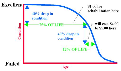
Figure 1. Pavement condition life cycle.
