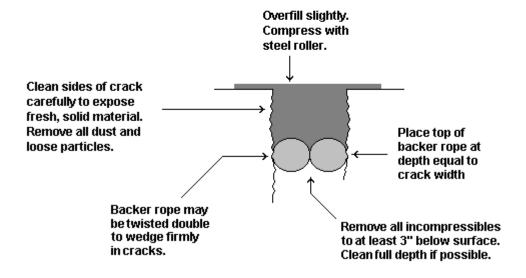
Figure 3. Overband sealing.
